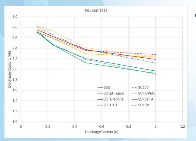
After previous tests (C20, 2 Reserve Capacities, gassing and qDCA), clearly 3BS pastes (3BS, Van A and HT-1) showed lower capacities in higher discharge current than other 4BS pastes (SC100, SC+pHagent, SC+ $\beta$ -PbO, SC+Graphite, SC+carbon black). This probably means larger pores in those 4BS plates is advantageous for high power performance.
