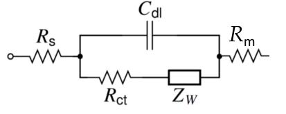
Total resistance =  $R_s + R_{ct} + Z_w + C_{dl} + R_m + Z_w$  (Warburg element) =  $A_w/(j\omega)^{0.5}$
