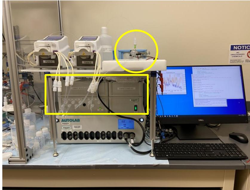
*Microfluidic cell + in line reference electrode for active material deposition + testing*
