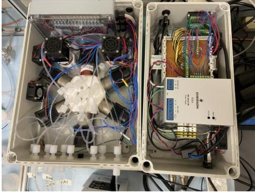
*Overview of E-SMART automated system, with 8 independent pump and valve channels for 6 MEM solutions and 1 rinse and 1 deposition solution*
