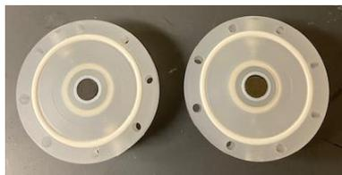
Top view cross section of flow cell with glassy carbon RDEs
